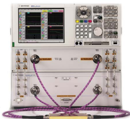
2-port PNA network analyzer utilizing the 2-port N4420B Test Set.
